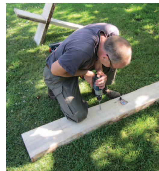
'Vlad the Impaler' drills out the corners of the 'letterbox' on the back of the stool. It helps to get the fit as tight as possible for rigidity
