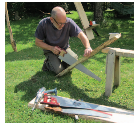
Cutting the shoulders on the seat piece with a Pax rip saw, made in Sheffield by Thomas Flinn
